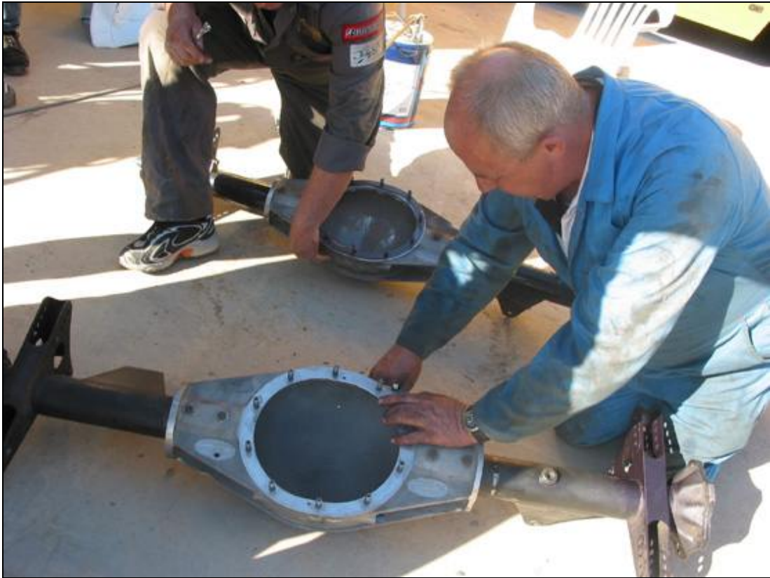
Above: The team prepares the replacement diff housing
